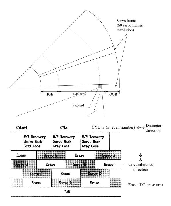
Figure 4.7 Physical sector servo configuration on disk surface
